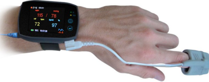
Fig. 5: SOMNOtouch NIBP, a cuffless solution for ambulatory blood pressure recording [27].
